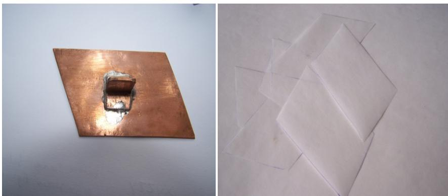
Once you have cut your supply of paper wraps you are ready to start wrapping. Slightly damp your finger to aid in the wrapping it will make it a lot easier to handle the paper. You can make a rolling jig, there are a number of designs out there to try, a simple one is a groove for the bullet to sit in and guide lines to aid in rolling straight.
