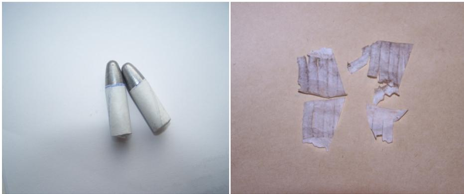
Once you have wrapped your bullets you must steam them for 3 - 5 seconds in a colander over the steam from a pan or a kettle, this will shrink and tighten the paper wrap and hold it in place, this is why glue is not required. Your bullets as they can now be called are ready to go in their shooting block or storage box ready for the trip to the range even if only one way it will protect them from damage.
