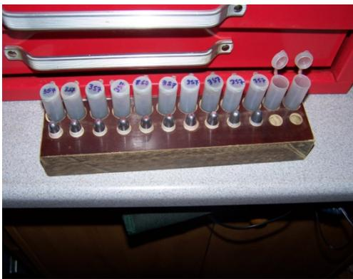
To help prevent loading errors a loading block is a good idea, a minimum of 12 rows are required 10 to count and two warmers into the bank, the design and make up is your preference but the minimum is space for phials and bullets, you can add rows for card wads or pins for caps.
