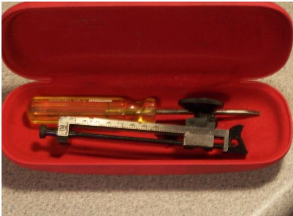
Rear Sight in travel case (Old glasses case is an ideal item as they come in a plastic bag) with fitting tool screwdriver and allen key, sights are precision instruments and must be protected for travelling and storage to prevent damage.
